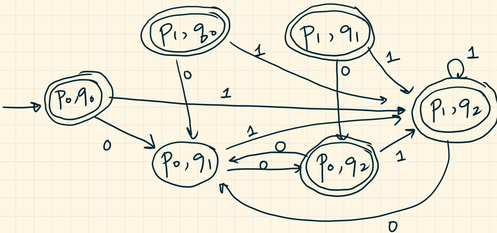
Transition function  $\delta : (P \times Q) \times \Sigma \rightarrow P \times Q$
