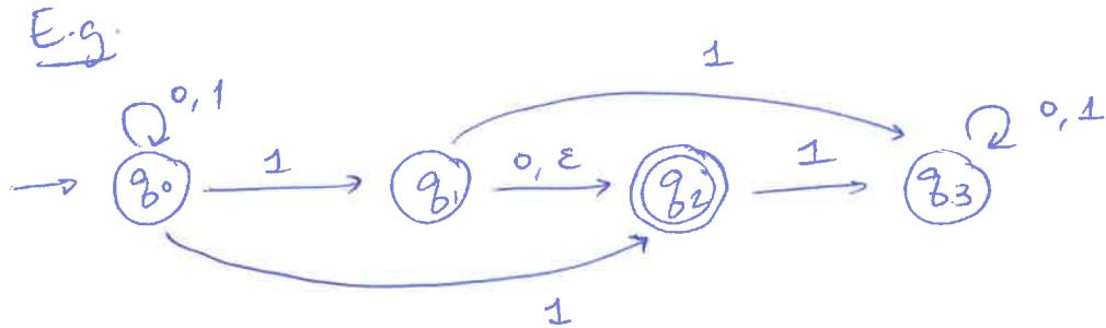
Calculation tree example :  $w = \underline{1} \underline{1} 0$
